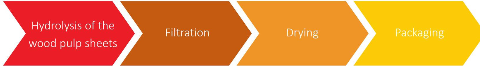
1. Sheets of wood pulp are added to glass lined reactors, for hydrolysis of the wood pulp which is carried out at the required temperature and pressure. The slurry then formed goes to the Quality Division that tests the nature and texture of the slurry.
